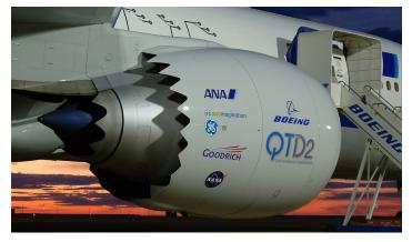
Figure C: Final chevron shapes—asymmetrical—in place on engine casing and nozzle.
