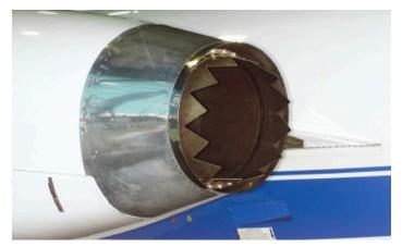
Figure B: An early chevron test article inside an engine nozzle.
